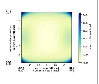
spot diameter at 86.5% level for a Gaussian beam (M² = 1) with 30.0 mm diameter at  $1/e^2$ , clipped at 30.0 mm field size and mirror distances as given above for a two mirror scan system
